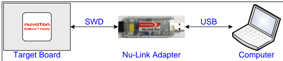
Figure 4-1 Nu-Link Adapter Connection Diagram
